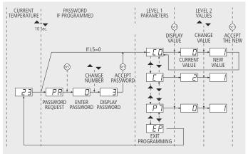
**REMARK:** If no key is pressed for 25 seconds in either of the previous steps, the controller will automatically return to the current temperature display status without modifying any of the parameters values.
