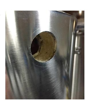
tun. Then go ahead and drill the outer hole, paying close attention to stop applying pressure once the outter hole is cut. Be sure to firmly grasp or secure the mash tun, and put your power drill on the highest speed setting for the cleanest cut.
