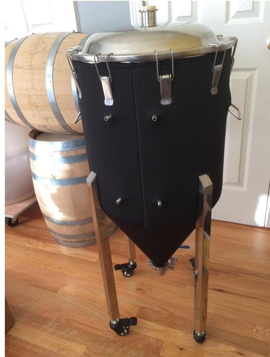
When removing the jacket, pull the neoprene out from around the barbs carefully. As you can see from the photo to the right, the holes in the neoprene do not rip and it holds up nicely!
